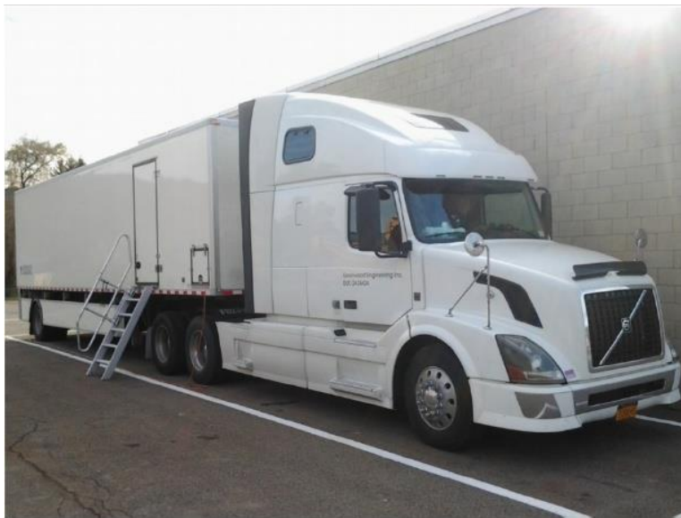
Figure 1.6 Traffic Speed Deflectometer Device (TSDD) used in the pooled fund study TPF-5(385)
