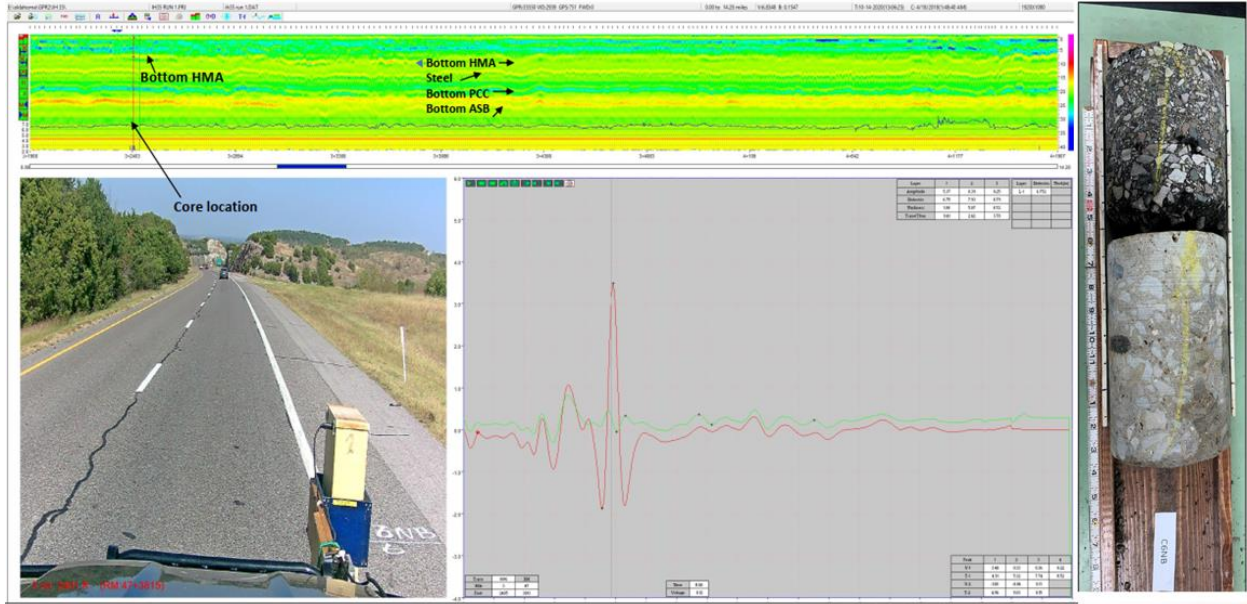
Figure B.3 Location of Core 6 from ODOT survey on I-35
