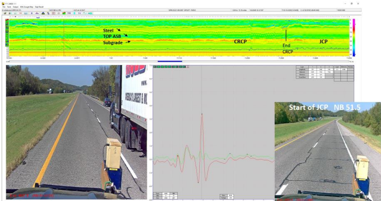
Figure B.4 Inside lane at transition from CRCP to JCP @ Mile Post 51.5 on I-35
