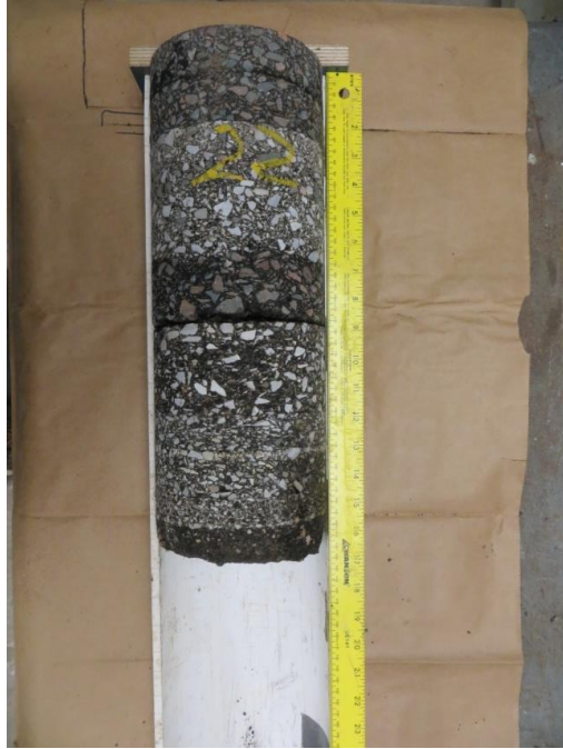
Figure A.13 Core #22 on SH-7
