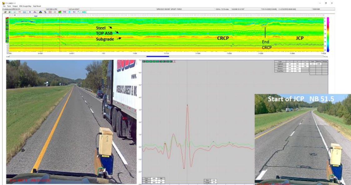
Figure 2.2 GPR and video images from north-bound I-35 section near Mile Post 51.5
