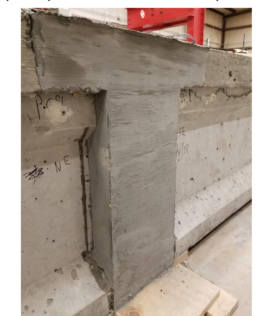
New Construction Continuity Joint with Positive and Negative Moment Reinforcement (Above) and Finished UHPC Joint (Below) Retrofit Construction Continuity Joint with Positive and Negative Moment Reinforcement (Above) and Finished UHPC Joint (Below)
