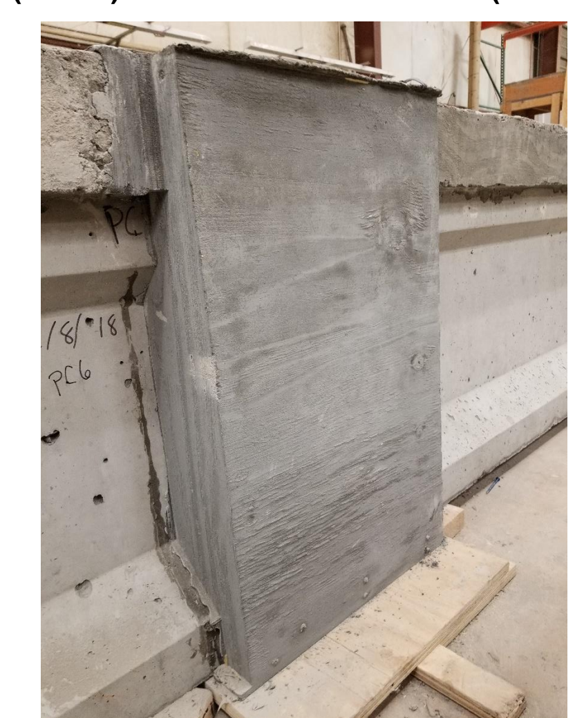
New Construction Continuity Joint with Positive and Negative Moment Reinforcement (Above) and Finished UHPC Joint (Below) Retrofit Construction Continuity Joint with Positive and Negative Moment Reinforcement (Above) and Finished UHPC Joint (Below)
