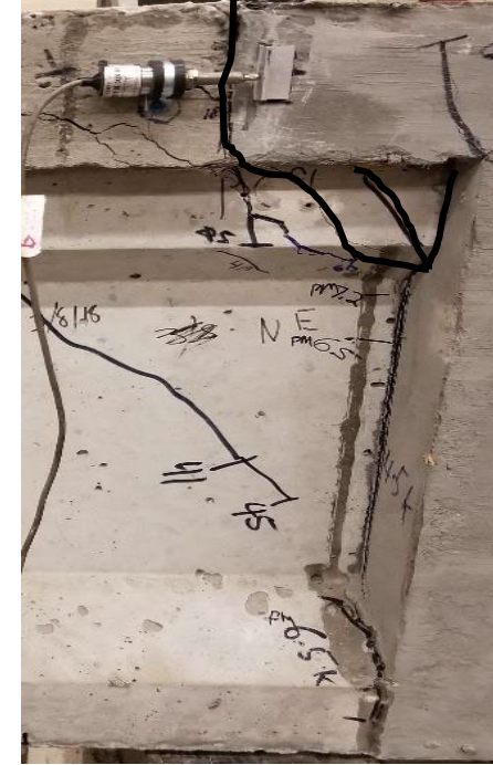
Flexural and flexure-shear cracking at joint interface
