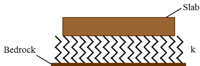
Figure 2. Slab on Winkler Foundation
