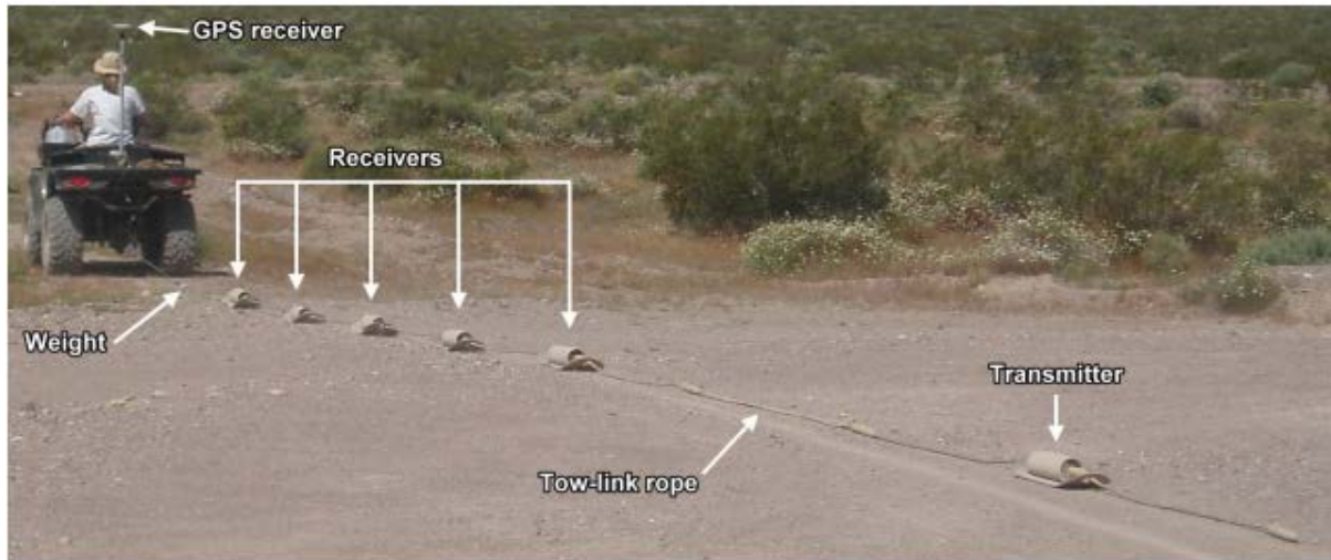
Figure 2-1. The OhmMapper system shown with five receiver dipoles and the transmitter dipole towed by an all-terrain vehicle (Lucius et al. 2008) (5)
