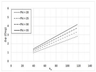
Effective Aspect Ratio vs. Change in Friction Angle
