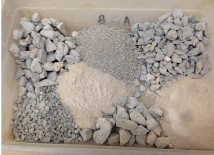
Figure 2.7a: Shows the coarse gradation in containers before the addition of moisture.
