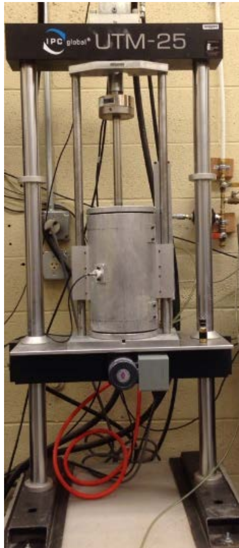
Figure 2.5: UTM-25 utilized for the application of various stress paths on laboratory specimen.
