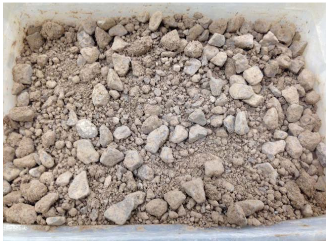
Figure 2.8a: Material after the addition and mixing of water for the coarse gradation.
