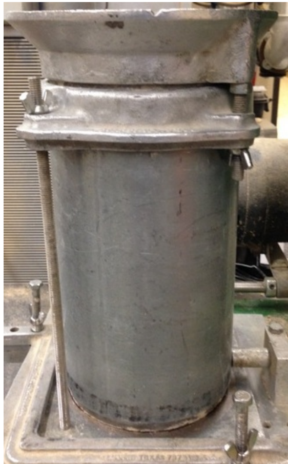
Figure 2.3: Shows the cylindrical mold utilized for the specimen generation.
