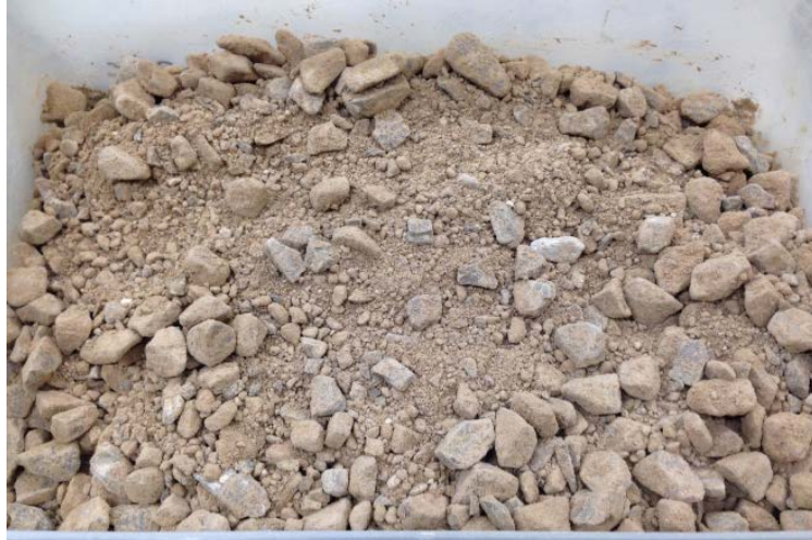
Figure 2.8b: Material after the addition and mixing of water for the intermediate gradation.
