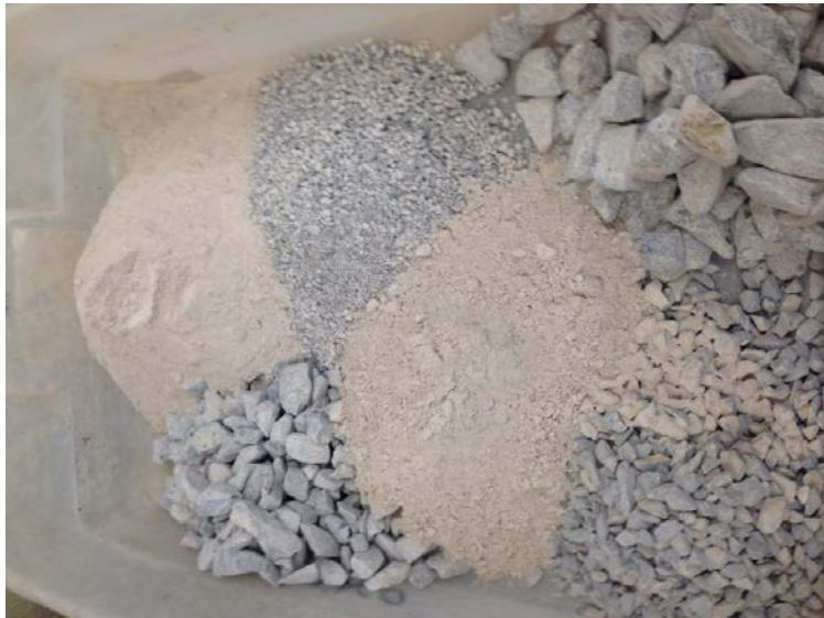
Figure 2.7b: Shows the intermediate gradation in containers before the addition of moisture.
