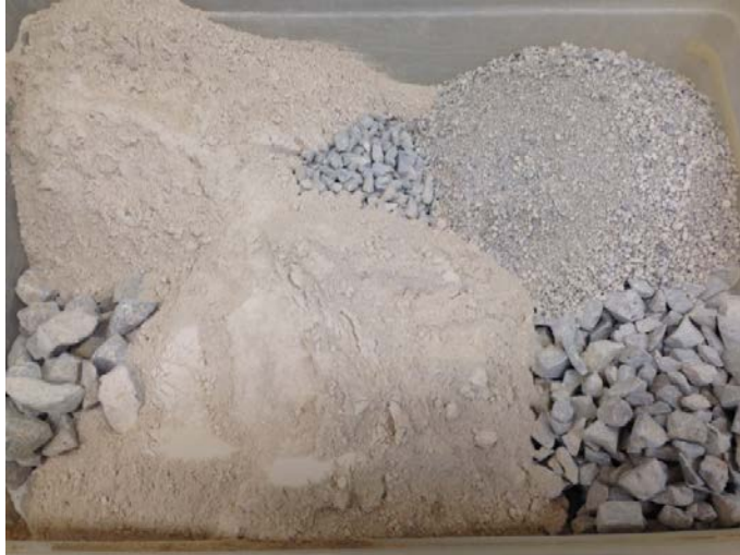
Figure 2.7c: Shows the fine gradation in containers before the addition of moisture.
