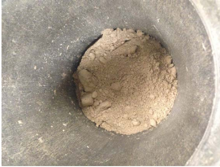
Figure 2.9a: Shows the process of compaction of loose material in the first layer
