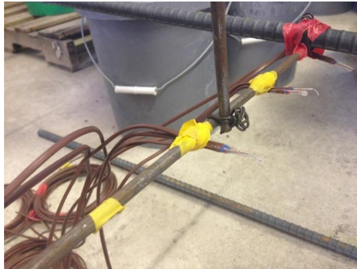
Figure 3.3 – Internal Type II thermocouples
