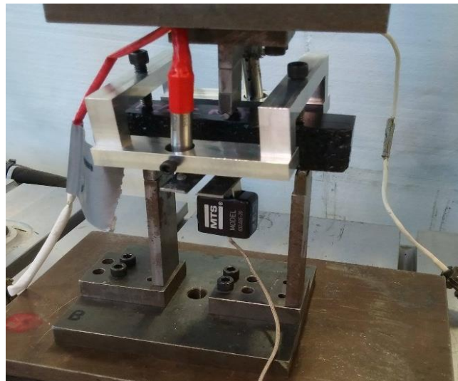
Figure 21: Initial load setup by the PI to examine the fracture toughness of PC
