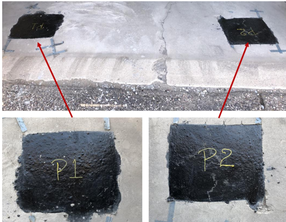
Figure 53: Two PC field samples after one year of weather exposure.
