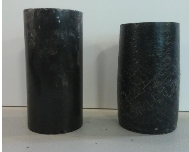
Figure 12: Compression cylinders: Tested sample (right) with untested (left).
