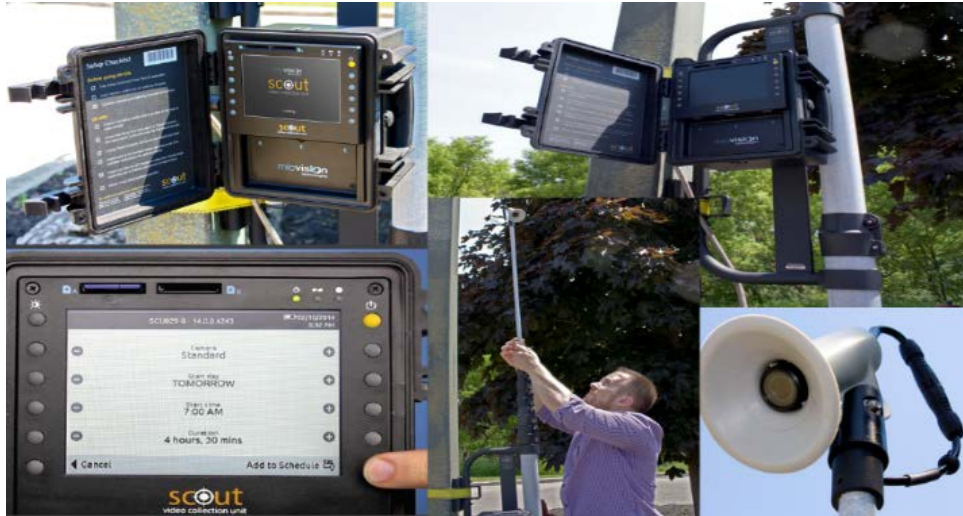
Figure 17 – Traffic camera (with all its components) purchased and being used in transportation and traffic engineering classes at Louisiana Tech University.
