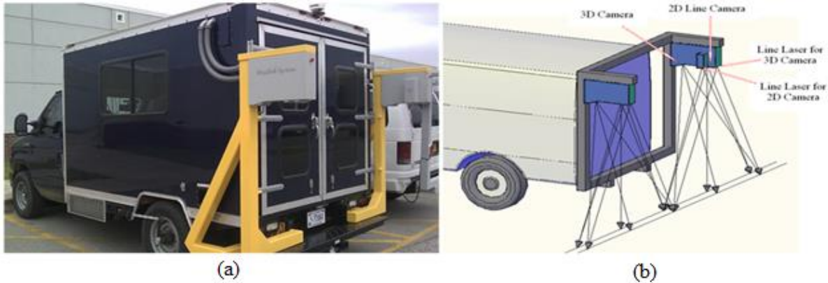
Figure 4 DHDV Vehicle (a) Exterior Appearance; (b) Working Principle
