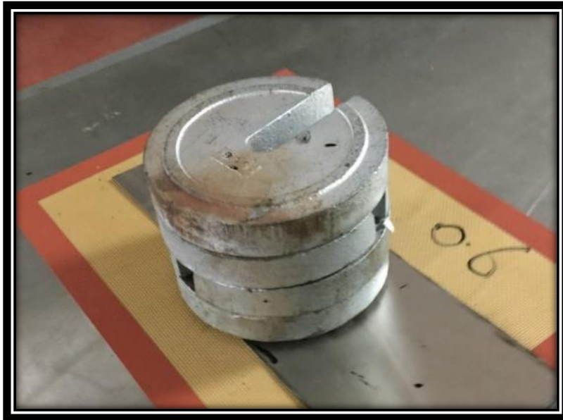
Figure 131. The loads placed over the thick glass
