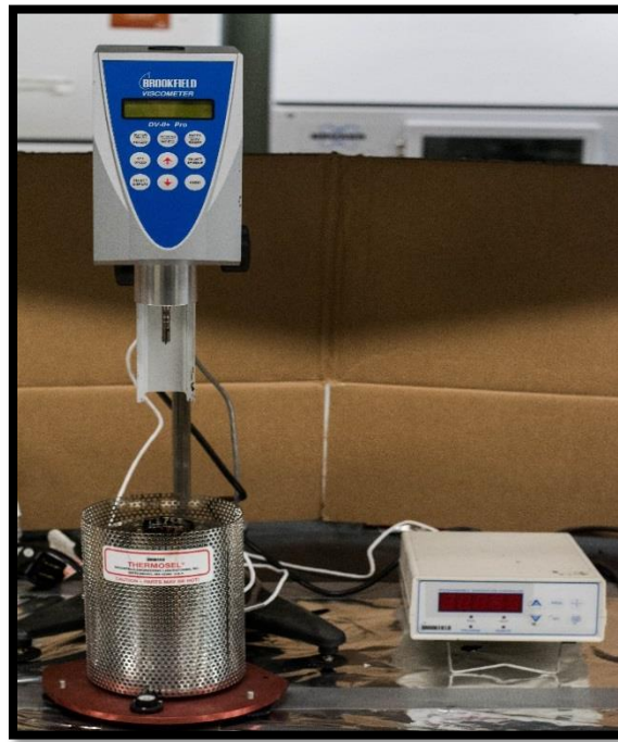
Figure 17. A DV-II+ Pro Rotational Viscometer (RV)
