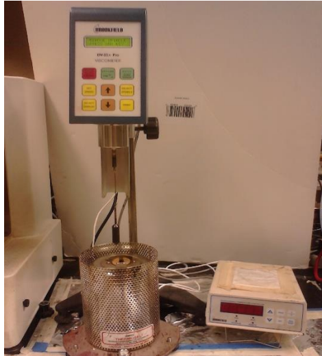
Figure 65. Rotational Viscosity test setup for asphalt binder
