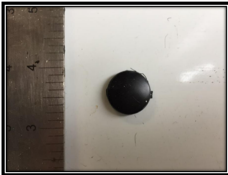
Figure 127.The binder was removed from the silicon mold
