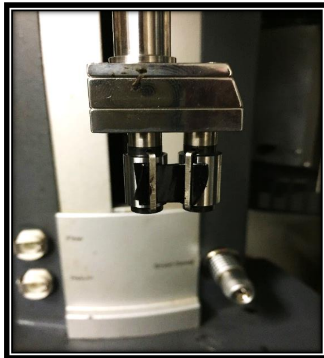
Figure 141. SER fixture after loading the sample
