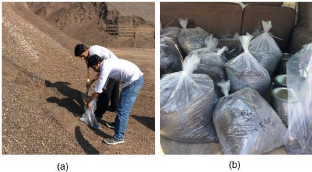
Figure 62. (a) Collection of aggregates for laboratory produced asphalt mixes; (b) collected aggregates and asphalt binder.
