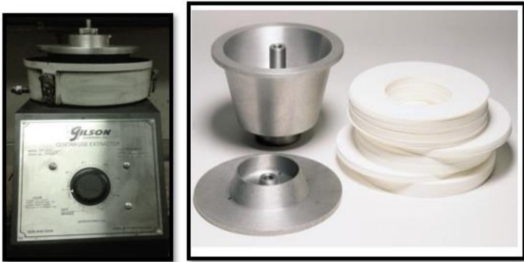
Figure 13. Centrifuge machine with extraction bowl and filters
