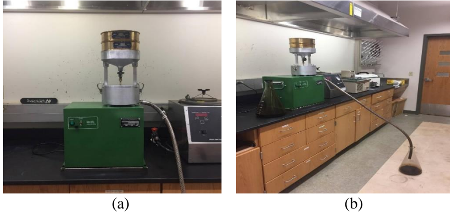
Figure 31: Binder solvent extraction in centrifuge phase II for removal of fines
