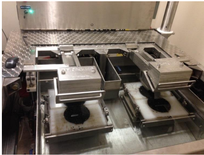
Figure 7: UNM Hamburg Wheel Tracking Testing
