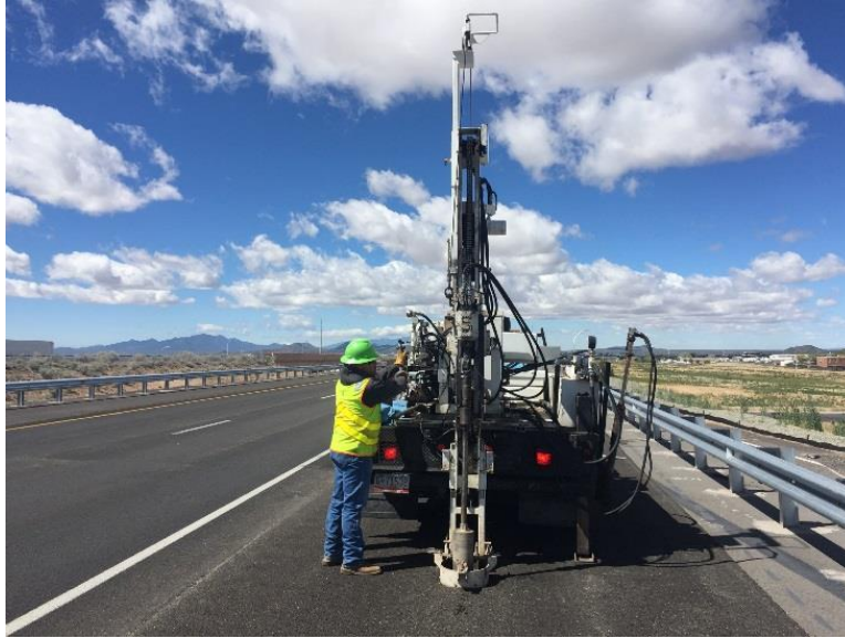
Figure 18: Field core collection from mixture 29 pavement test section location
