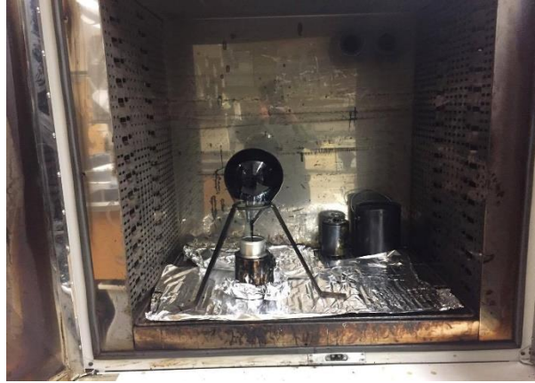
Figure 33: Asphalt binder recovery post-rotavapor process
