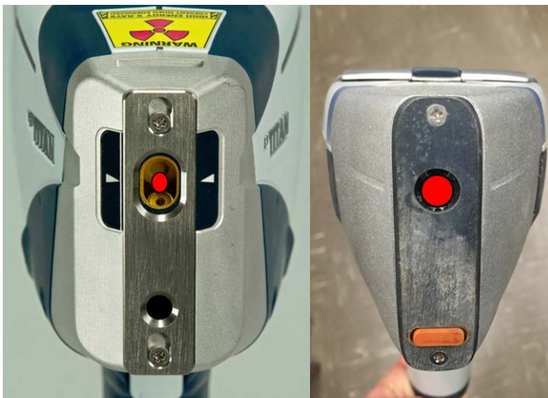
Figure 2: Beam footprint (red portion) of the S1 Titan (left) and Niton XL3t (right) PHXRF devices.
