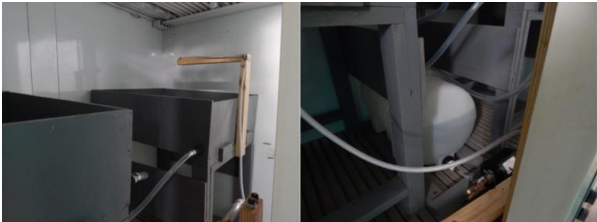
Figure 3.2: Rain simulation exposure setup consisting of two interconnected basins with spray nozzle and water reservoir below.
