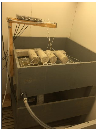
Figure 3.3: Samples placed in rain simulation setup.
