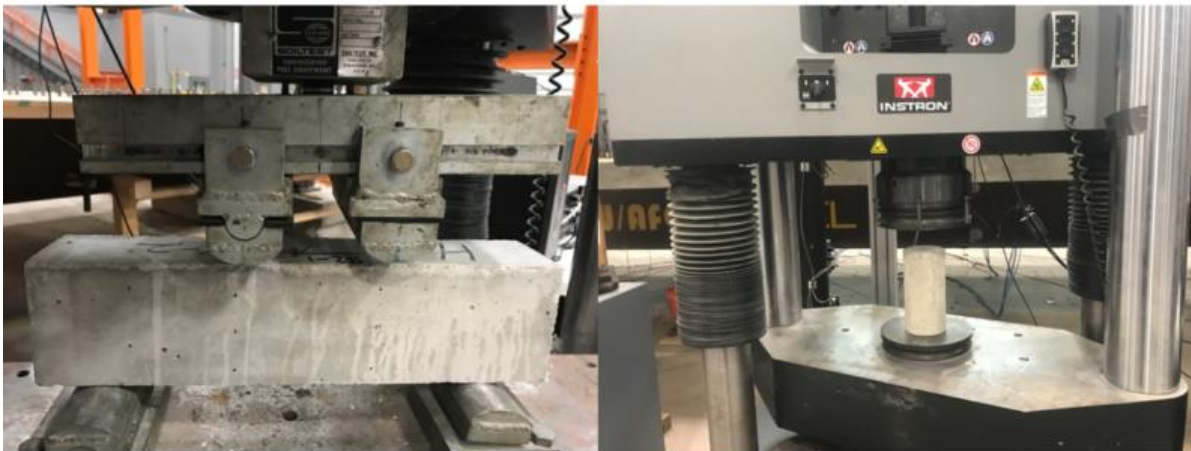
Figure 3-7: Experimental setup of third-point flexural strength test and compressive strength test on universal testing frame.
