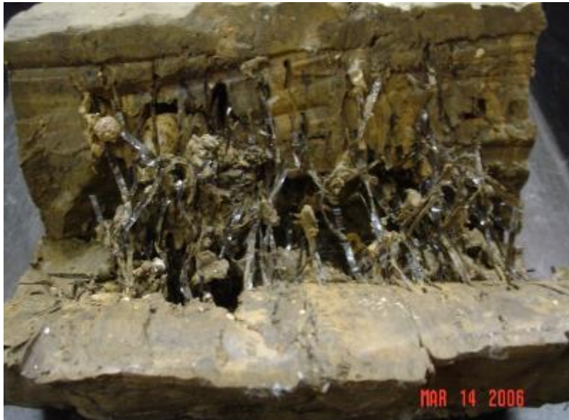
Figure 20. Dissected Field Specimen Following Triaxial Test (Gregory2006)
