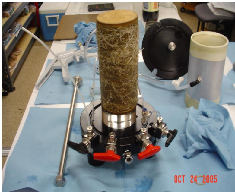
Figure 50. FRS Specimen Mounted on Base of Triaxial Cell (Gregory 2006)
