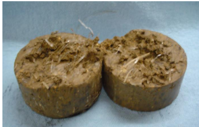
Figure 60. Dissected Direct Shear Clay Specimen with Exposed Fibers (Gregory 2006)
