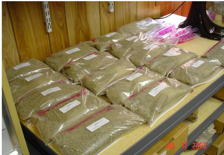
Figure 34. Clay Specimens Prior to Hydration (Gregory 2006)
