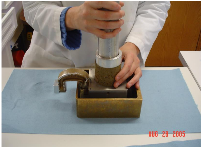
Figure 57. Mounting Direct Shear Specimen (Gregory 2006)
