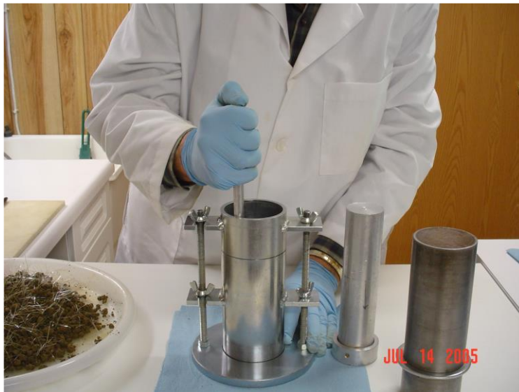
Figure 41. Rod Plunged to Near Bottom of Mold during Initial Compaction (Gregory 2006)
