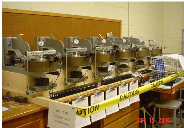
Figure 61. Direct Shear Creep Devices (Gregory 2006)
