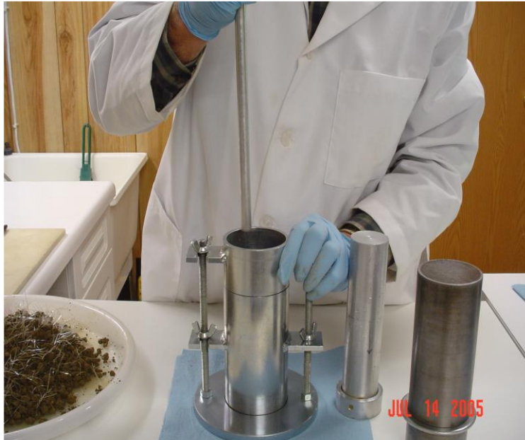
Figure 40. Compaction with a Metal Rod (Gregory 2006)
