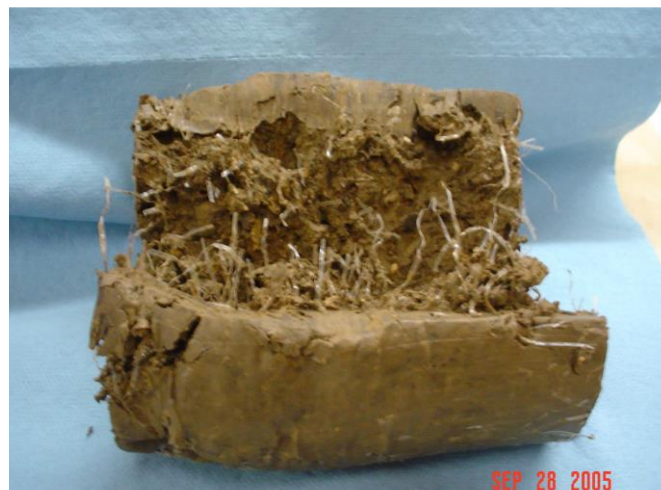
Figure 56. Dissected Triaxial Clay Specimen with Exposed Fibers (Gregory 2006)
