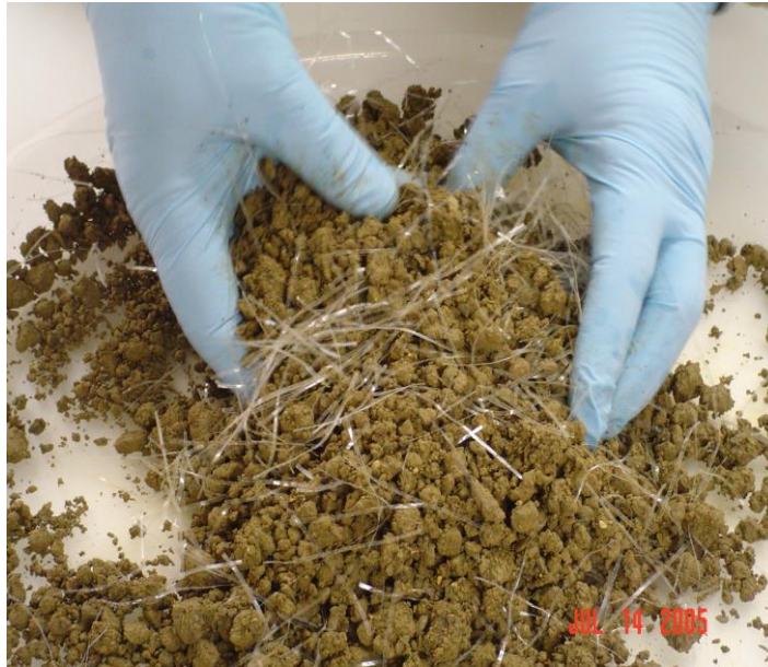
Figure 37. Final Hand Mixing of FRS Specimen (Gregory 2006)
