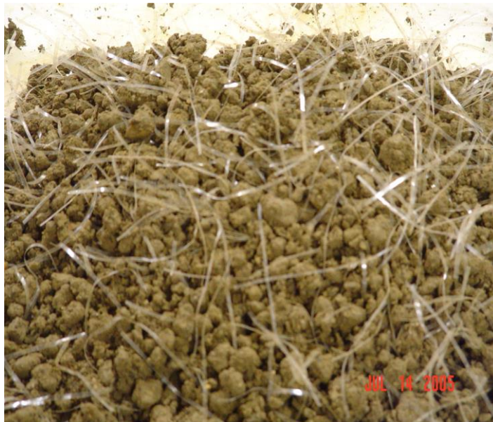
Figure 38. Mixed FRS Specimen Ready for Storage or Compaction (Gregory 2006)
