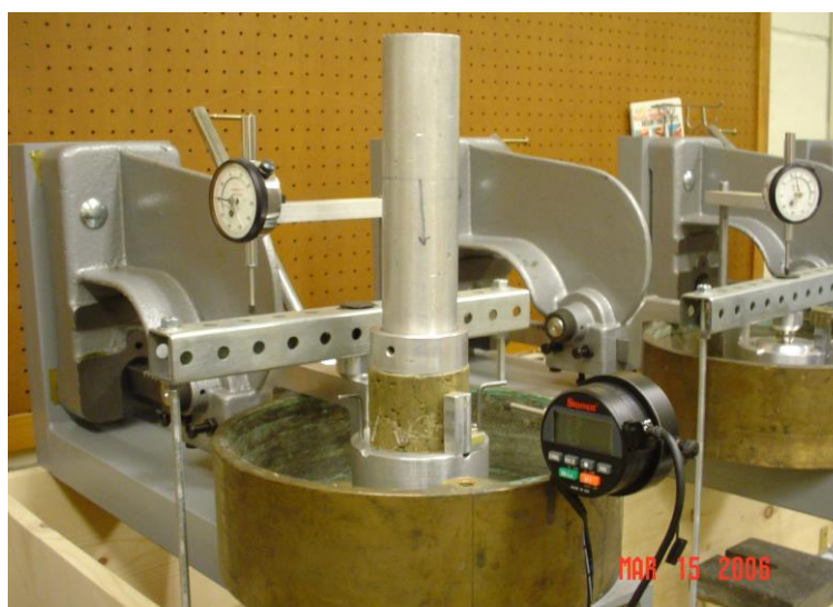
Figure 62. Mounting Clay Specimen in Creep Device (Gregory 2006)
