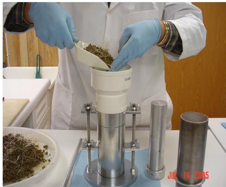
Figure 39. Placement of Loose Specimen into Mold (Gregory 2006)
