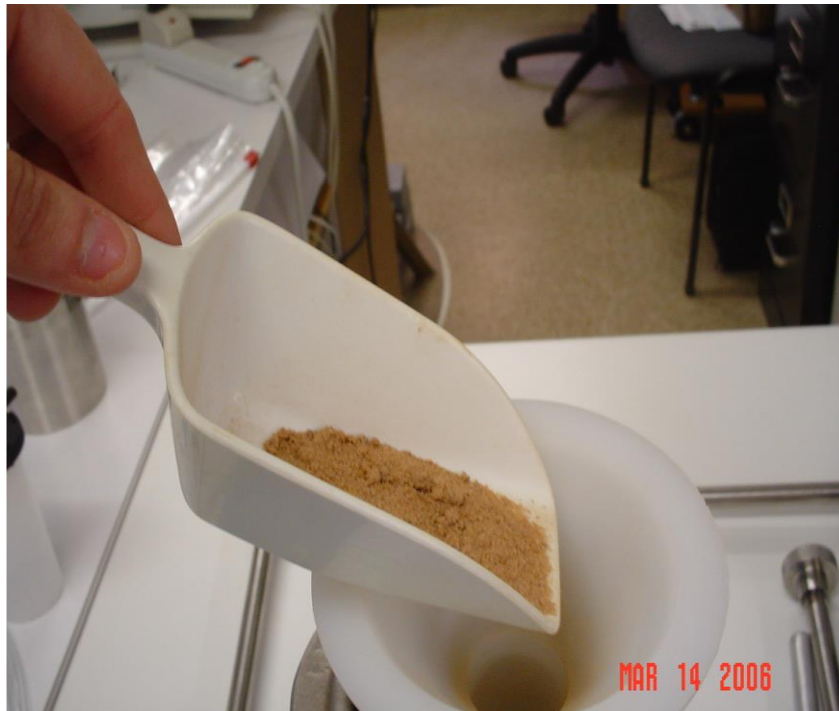
Figure 46. Preparation of Sand Specimen in Split Mold (Gregory 2006)
