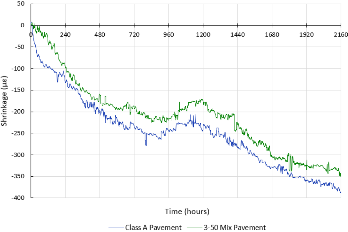
Figure 10-14. Pavement Panel Shrinkage Comparison of Class A and 3-50 Mixes
