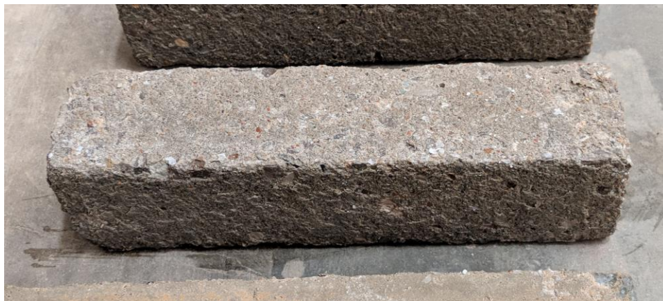
Figure 9-7. Mix 2-20 Specimen at 304 Freeze/Thaw Cycles
