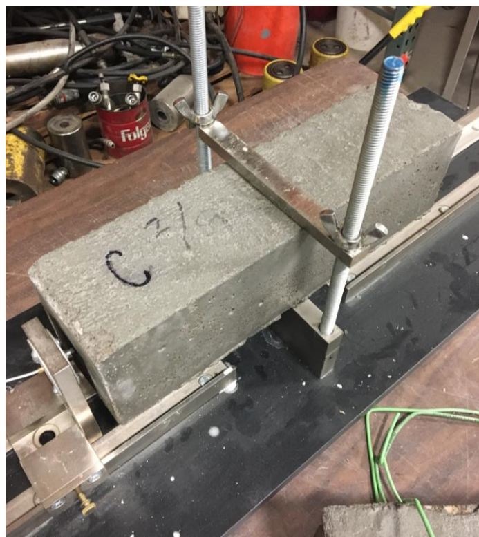
Figure 9-2. Longitudinal Dynamic Modulus of Elasticity Test Setup
