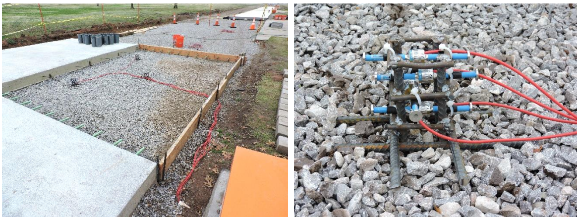
Figure 10-11. VWS Gage Layout (l) and Close-up of Tree No. 1 (r) for Panel No. 8
