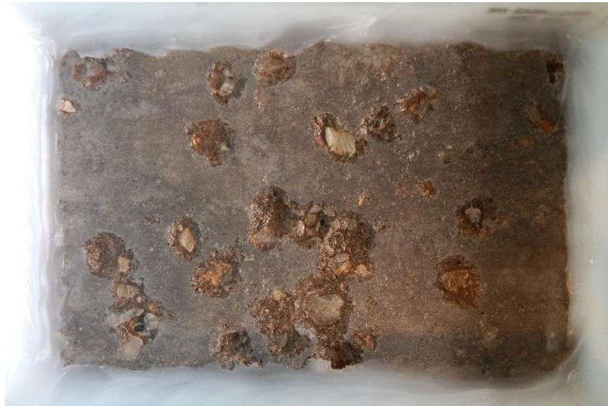
Figure 6-18. 75 Percent RCA Specimen After 50 Cycles
