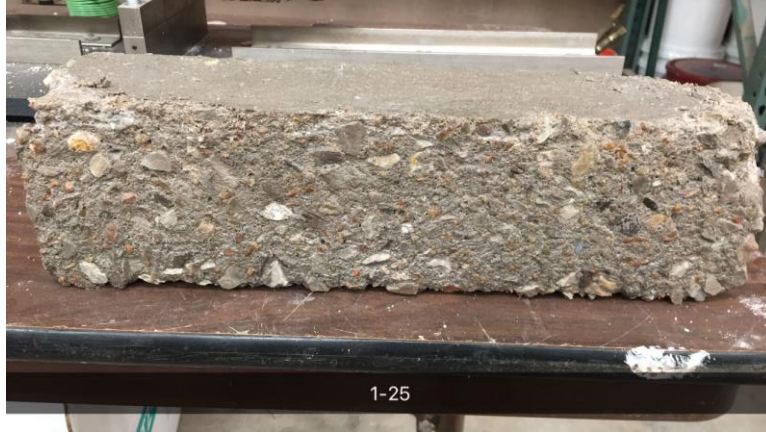
Figure 5-9. Mix 1-25 Specimen at 304 Freeze/Thaw Cycles
