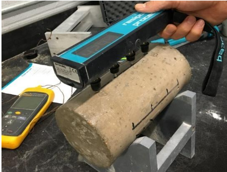
Figure 6-1. Surface Electrical Resistivity Test
