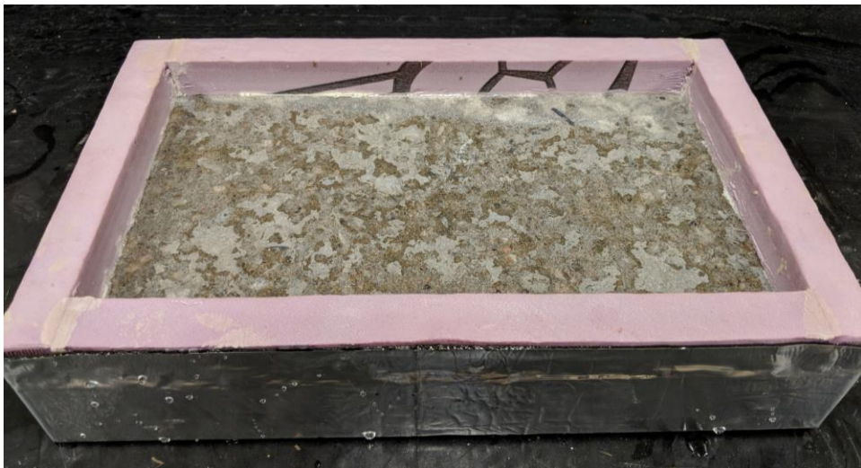
Figure 9-13. Mix 3-60 Salt Scaling Specimen at 50 Cycles
