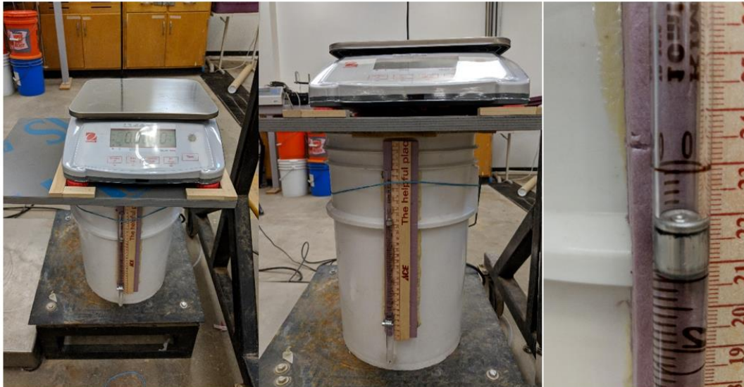
Figure 7-8. Hydrostatic Weighing Setup
