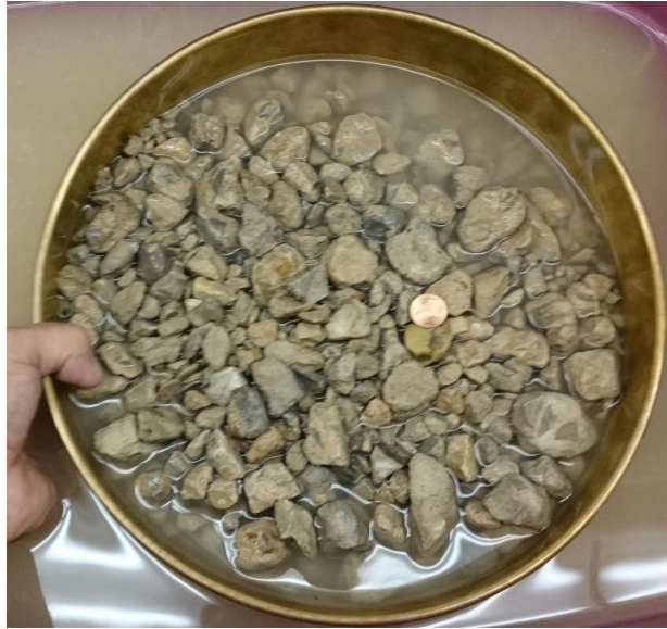
Figure 7-1. Washing of RCA Samples
