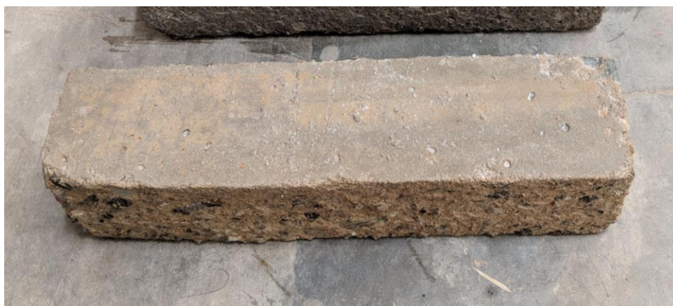
Figure 9-8. Mix 2-60 Specimen at 304 Freeze/Thaw Cycles
