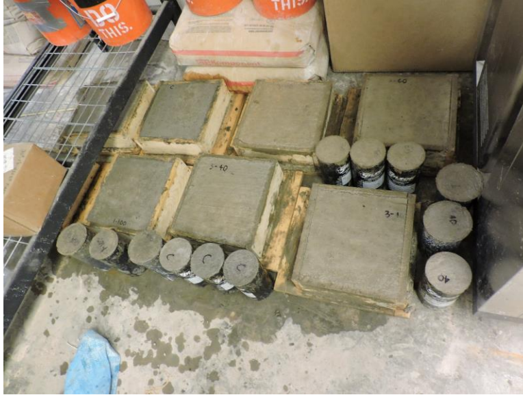
Figure 5-4. Salt Scaling Specimens as Cast
