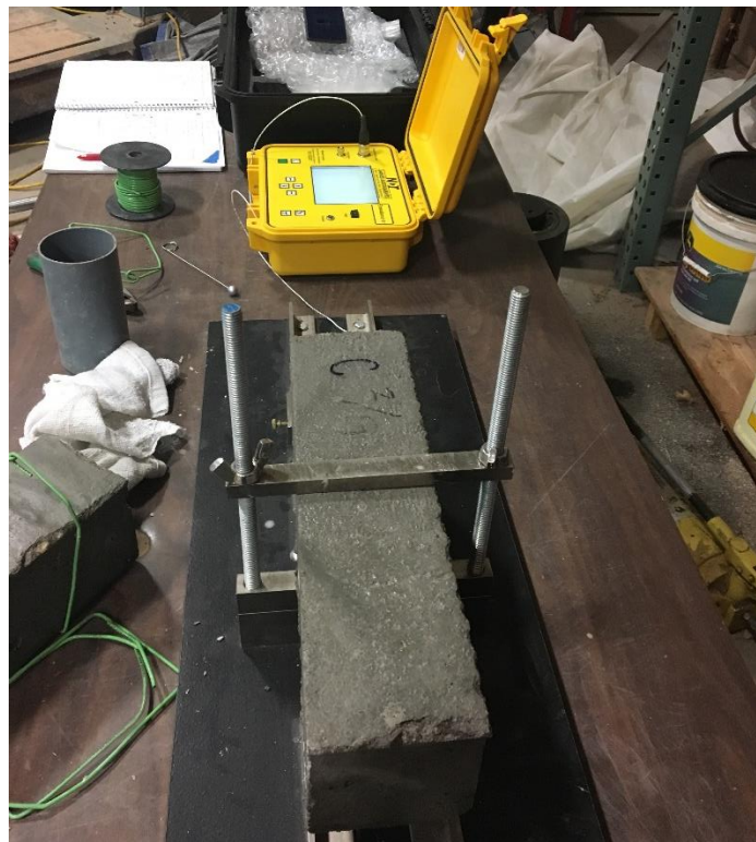
Figure 5-2. Longitudinal Dynamic Modulus of Elasticity Test Setup
