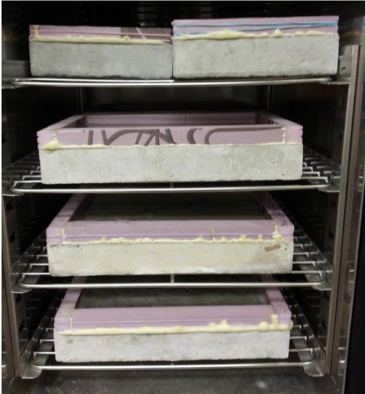
Figure 9-5. Salt Scaling Specimens within Environmental Chamber
