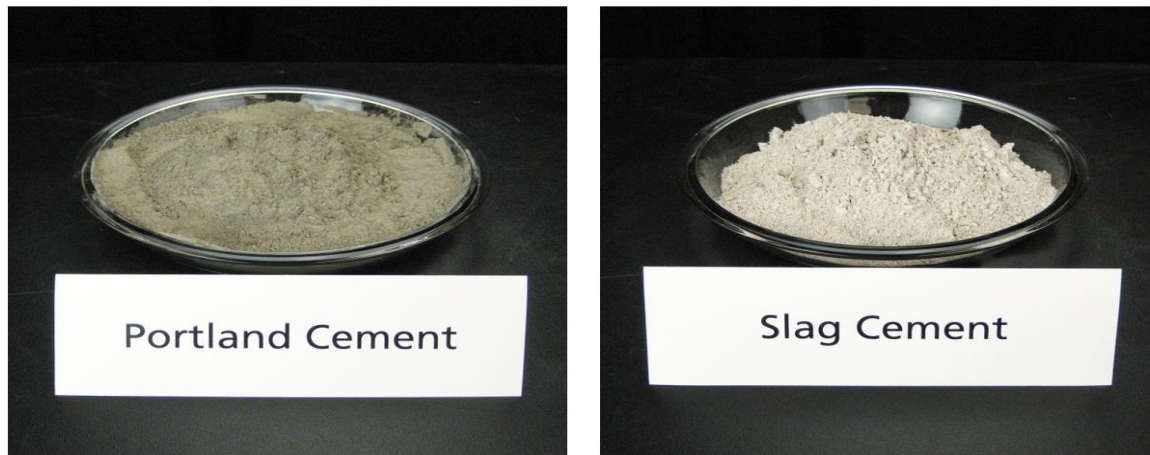
Figure 2-2. Physical Comparison of Portland Cement (left) and Slag Cement (right) (courtesy Slag Cement Association, 2019)
