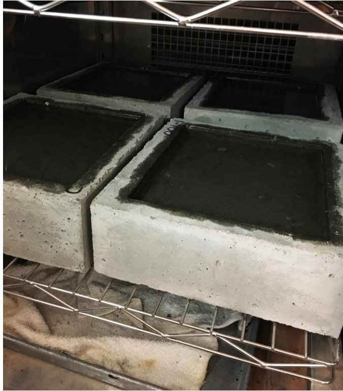
Figure 5-6. Salt Scaling Specimens within Environmental Chamber
