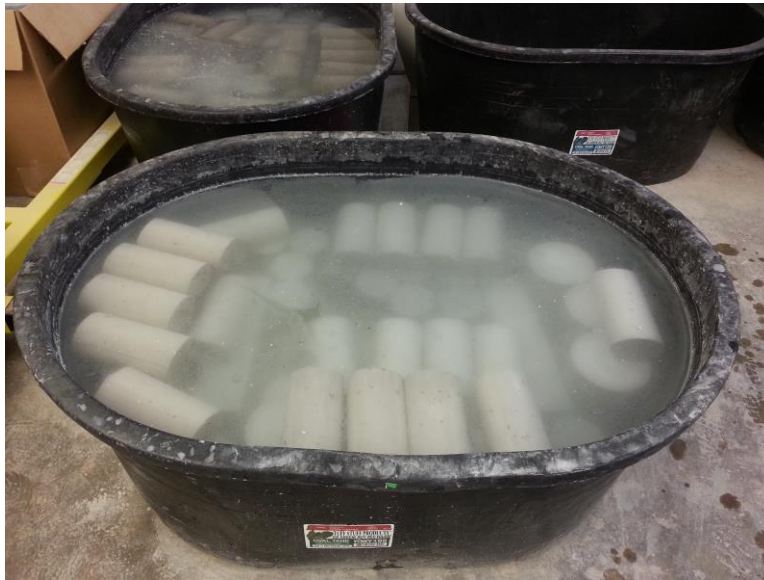
Figure 9-3. Constant Temperature Lime Water Tempering Tank
