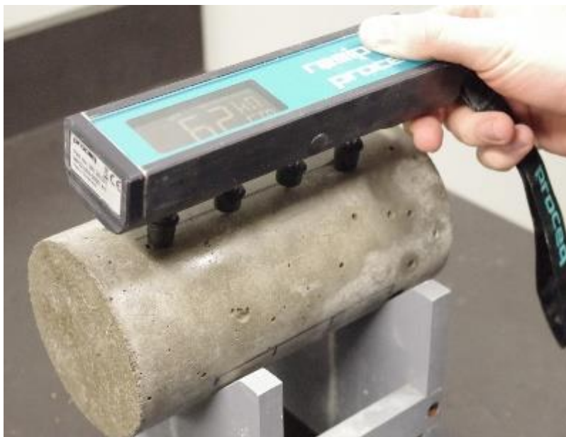
Figure 2-1: Example of surface resistivity test setup and resistivity probe.
